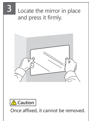
3 Locate the mirror in place and press it firmly.
