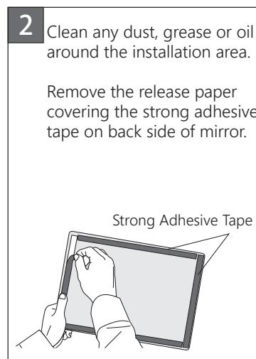
2 Clean any dust, grease or oil around the installation area.
